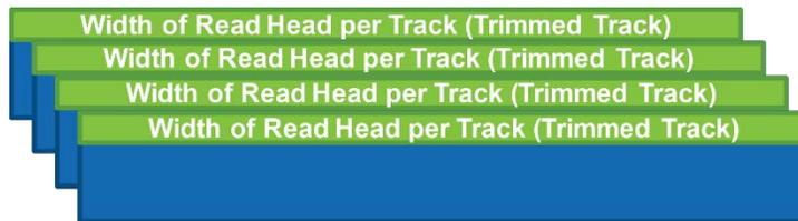
SMR drives do overlap tracks during writes to increase data density, which results in higher usable capacity.
