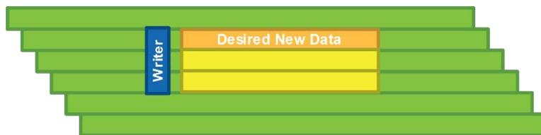
Deleting data from a band leaves holes, therefore garbage collection has to take place from time to time to clean up bands in order to allow new data to be appended at the end of the band. This process is similar to flash-based SSDs, although it occurs for a different reason.
