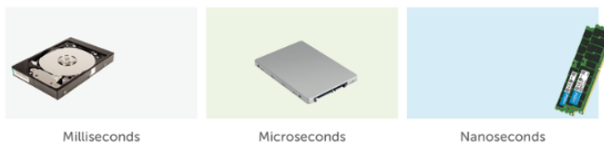
Latency comparison How much time does it take for data to get to the CPU?
